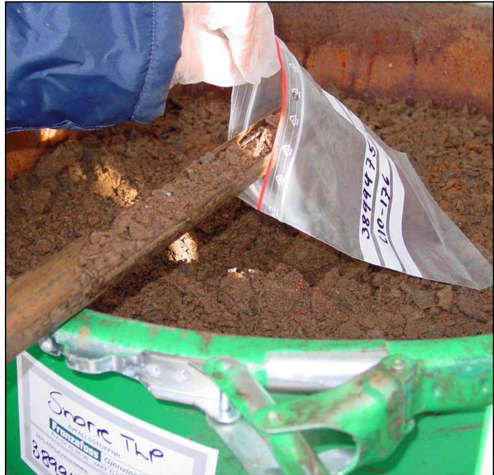
Sampling of typical LSA scale containing separator mass.
