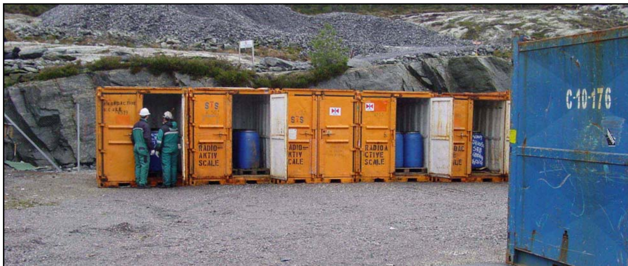
Temporary LSA scale storage at oil service base.
